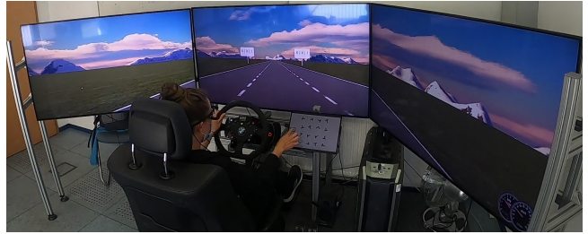
Figure 3: Driving simulator setup overview showing the lane-changing task and the secondary visual search task.
