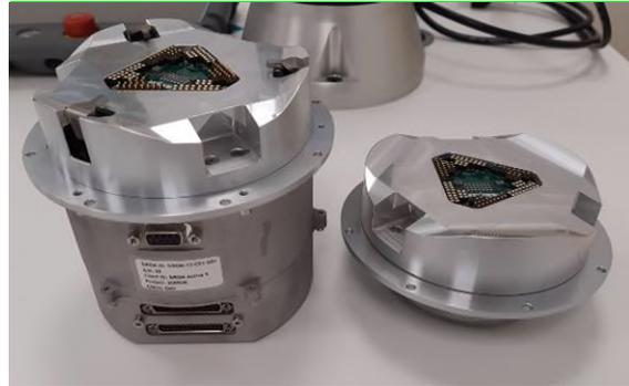
Figure 7: Active SIROM (left), Passive SIROM (right). PERIOD benchmarking versions
