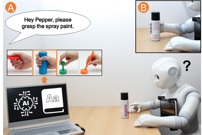
Fig. 1. Demonstrates conceptually how a Pepper robot successfully learns how to grasp an unknown object using an anthropomorphic end-effector.
