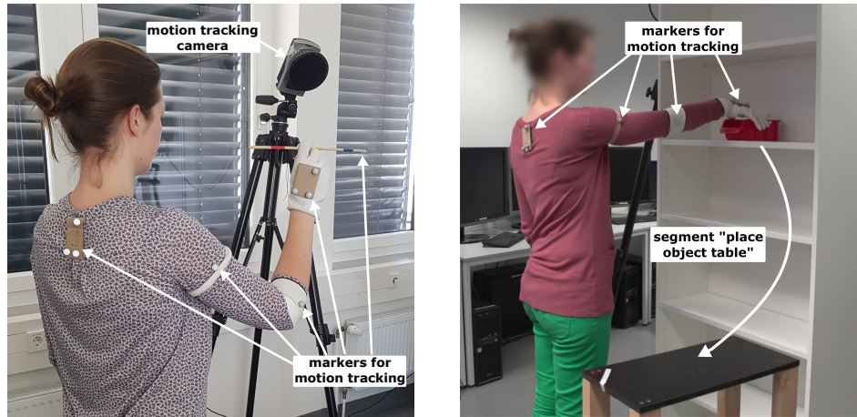
FIGURE 3. Setups for movement recordings. Left: Setup for stick-throwing recordings. (Image extracted from [23].) Right: Pick-and-place task, in which a box is grasped from a shelf, placed on a table, and vice versa. (Image adapted from [24].)
