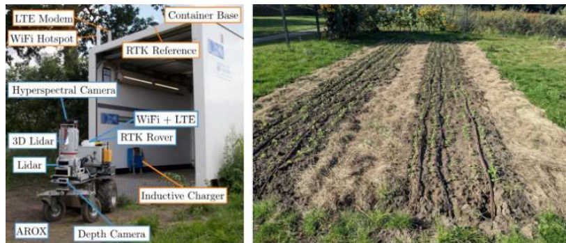
Fig. 1: (a) AROX platform and base station [Ho20] (b) Test plot for canola monitoring
