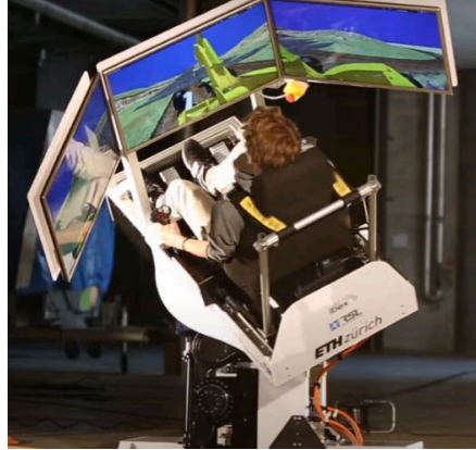
Fig. 2: The ETH teleoperation system can provide a user experience similar to a real excavator cockpit. Picture source: https://ibex.ethz.ch/
