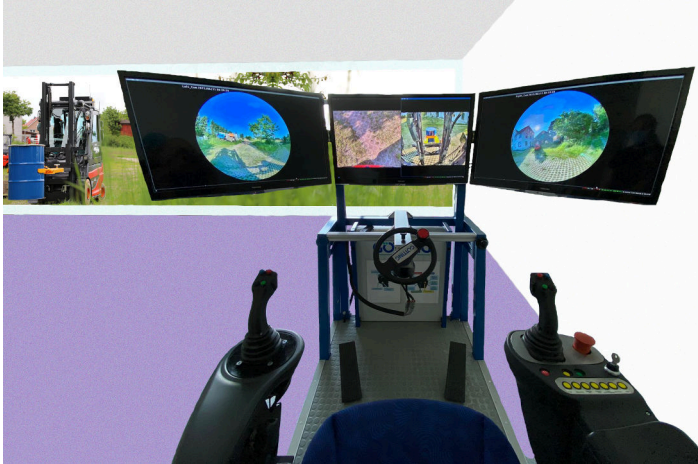
Fig. 3: Teleoperation of a forklift via Götting Control Station
