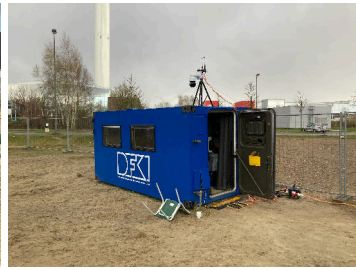
(b) In Operation with surveillance Camera and Antennas on the roof
