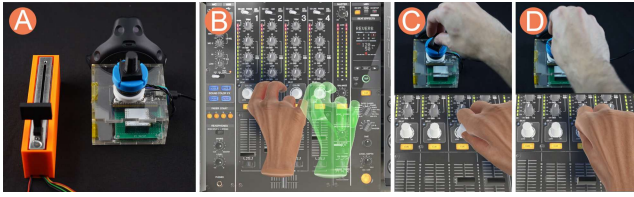
Figure 9: (A) displaying Feick et al. [21]’s slider proxy next to our knob proxy. (B) shows a user’s hand is redirected. (C) indicates the start position, while (D) shows the position of the hand after rotation in the real and virtual world.
