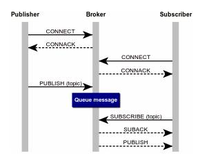
Figure 3. MQTT sequence diagram
