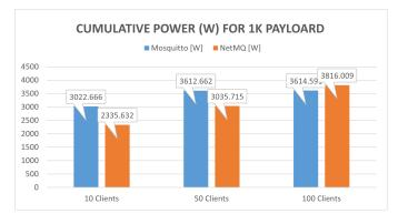
Figure 7. Comparison of power consumption in watt
