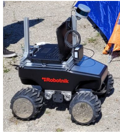
Figure 4. A Summit-XL with a preliminary sensor setup. (Photo by C. Rachuy.)
