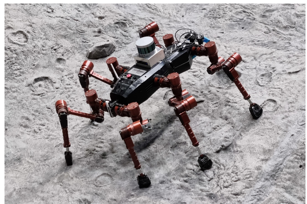
Figure 2. The six-legged walking system CREX on an artificial lunar crater. (Credit: DFKI, Annemarie Popp)
