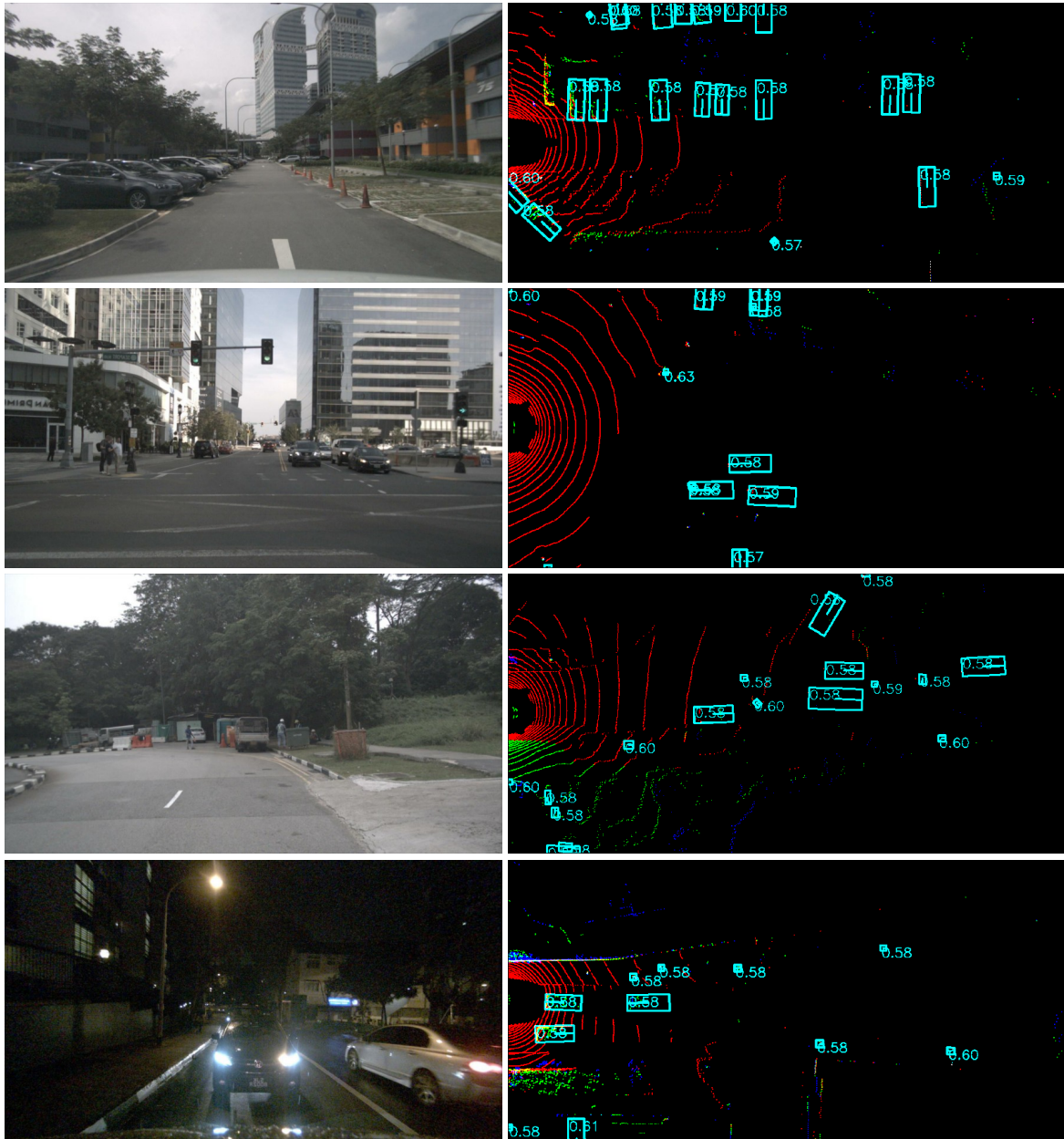
Figure 5: Visualization of the BEV detections predicted by our model. The model has good prediction for most cars, but has difficulties at the edges of the BEV lidar. It cannot detect all construction workers in image three, however construction workers are underrepresented in the dataset. At night the detection of the cars is very good despite the low visibility.
