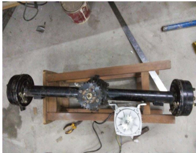
Fig. 1 Actual diagram of Differential mounted with 48V Brushless DC motor
