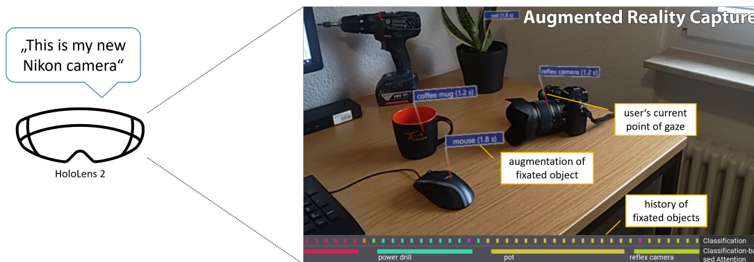
Fig. 8. Our prototype based on Microsoft’s HoloLens 2 classifies and augments fixated objects in real-time [Barz et al. 2021b]. It displays classification labels and the duration of recent attention events to the user as a hologram. The demo video can be viewed here: https://www.youtube.com/watch?v=bdNCIVz9yIE . In No-IDLE, we plan to enable interactive model adaptation based on foundation models: For instance, the user could create a specific instance of "reflex camera" and name it "Nikon camera" via speech (as shown in the image). This is related the COPDA project which aims to establish and maintain object relations like ownership. Other examples include that users may correct wrong classifications or teach new classes to the ML system in a mixed-initiative dialogue.
