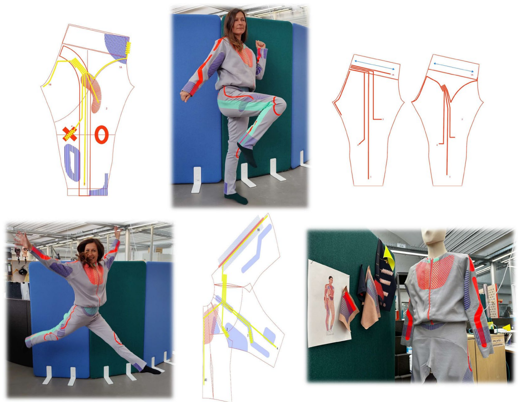
Figure 6. Design process of embedding the capacitive sensing technology into a custom-built suit by a professional experienced fashion designer.
