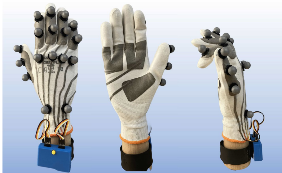
Figure 9. The capacitive glove is equipped with 8 capacitive channels, an additional 17 markers for the ground truth tracking, and the DAU worn on the wrist.
