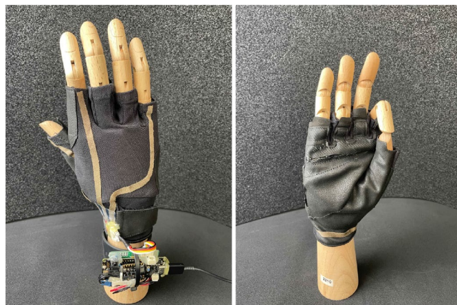
Figure 7. Gesture recognition glove with capacitive sensing and IMU. The wristband hosts the embedded board to realize real-time and on-the-edge (RTE).
