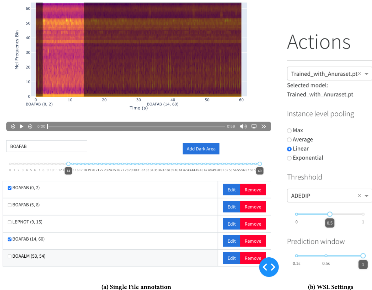
Figure 2: Annotation pane: Upon file upload, the model annotates the file with the detected species’ calls and onset, offset time. The user can modify the predictions if necessary (a) using UI components such as slider, buttons and input fields. The more experienced machine learning practitioner can adjust the post-hoc parameters of the weakly supervised setting to achieve the best performance such as pooling function, prediction threshold and the precision of the prediction window for the onset-offset times (0.1 - 1s)(b).
