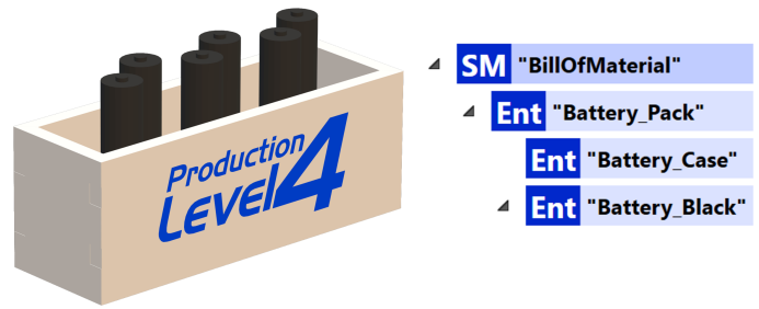
Fig. 4. The battery pack including 3D-printed black model batteries and the respective Bill-of-Material of the Battery Pack.
