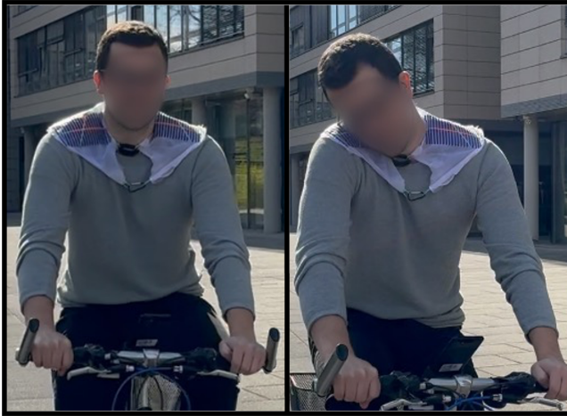
Figure 3: A participant of our data collection experiment executing a gesture by tapping the shoulder patch with his cheek while biking.
