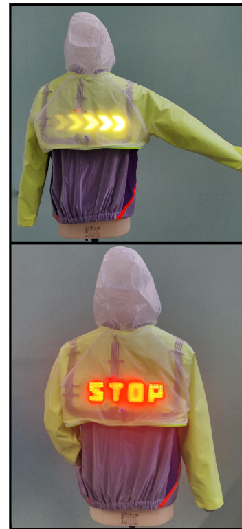
Figure 6: LED matrix attached to the rider’s back as a visible actuator to utilize shoulder tap input as an output to warn following cyclists.
