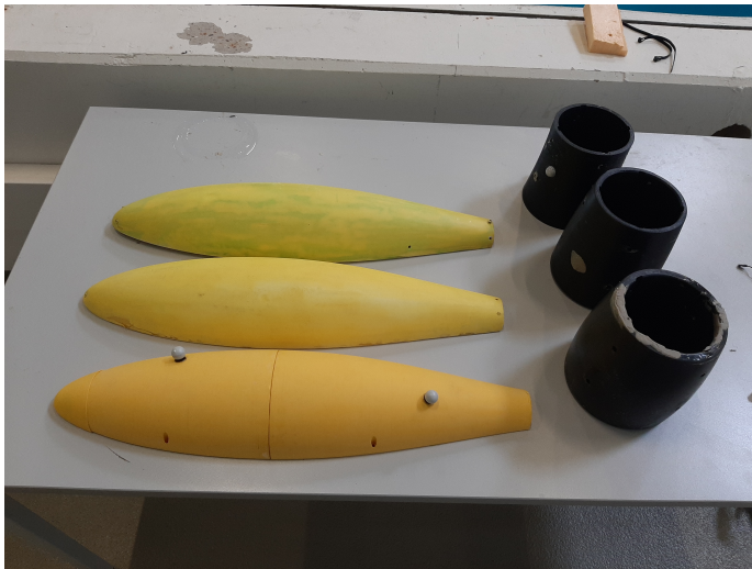
Fig. 14. Different versions of hulls in comparison. On the lower hull 3d tracking markers are visible.
