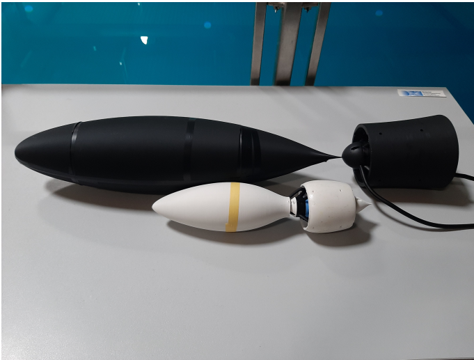
Fig. 2. First concept of AUV design as 3d prints.
