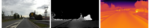
Figure 1. Three different modalities to perceive traffic scenarios in an automotive context. From left to right: Classical RGB, depth, and IR images from the InfraParis dataset [12].
