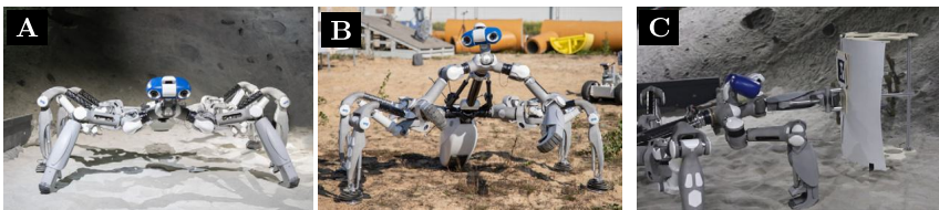
Figure 12.2 Mantis in its six-legged locomotion mode (A), four-legged manipulation posture (B), and five-legged transport mode (C). (Credit: Annemarie Popp, DFKI.)
