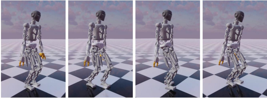
Figure 15.6 From right to left: RH5 Pedes executing a dynamic walk in a simulated environment using WBC.
