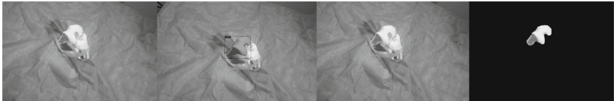
Fig. 2. from left: (1) original image; (2) detected segmentation and annotation; (3) polygon calculation; (4) calculated mask image
