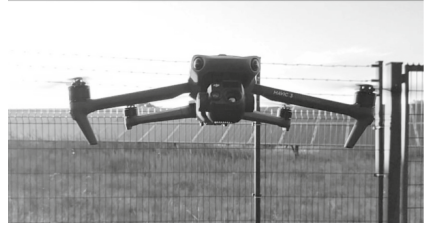
(b) DJI Mavic 3T drone used for thermal imaging and data collection in PV system inspections
