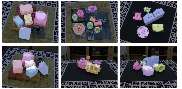
Fig. 11. Qualitative Result on T-LESS [39]. We render the objects with the estimated pose on top of the original images. The presented confidence scores are from the 2D object detection provided by BOP challenge 2023 [34]. Each column represents a scene captured from a different viewpoint. The visualizations demonstrate that our method is capable of effectively handling severe occlusion in cluttered environment.
