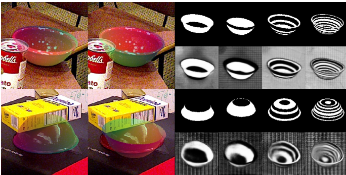
Fig. 13. Visualization of the YCB-V dataset. The first column is the ground truth, and the second column shows the estimated poses. The first example is a correctly estimated case, while the second example is one of incorrect estimation. The first and third rows on the right side show the ground truth of SymCode, while the second and fourth rows display the estimations. We found that under significant occlusion, the output binary codes still exhibit characteristics of a specific pose, although this pose is incorrect.
