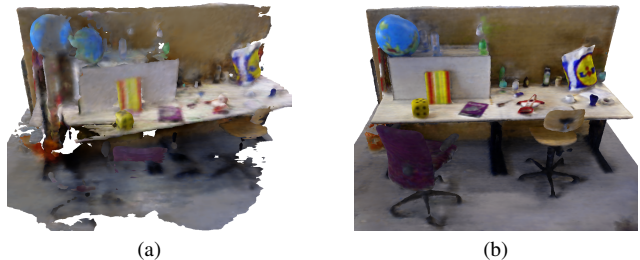
Figure 1. The reconstructed 3D mesh on the TUM RGB-D dataset [53], generated using our proposed method without uncertainty-guided reweighting and strategy, is illustrated in Fig. 1a. Conversely, Fig. 1b demonstrates the 3D mesh produced by our method after the incorporation of the uncertainty-aware strategy.
