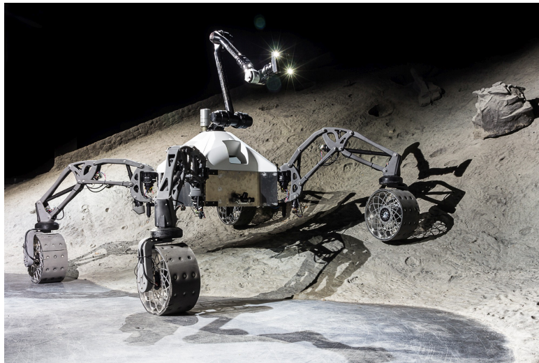
Figure 3.1: The SherpaTT robot is a planetary rover with an adaptable suspension system developed for planetary exploration. The picture shows the robot placed in an artificial crater environment at DFKI.
