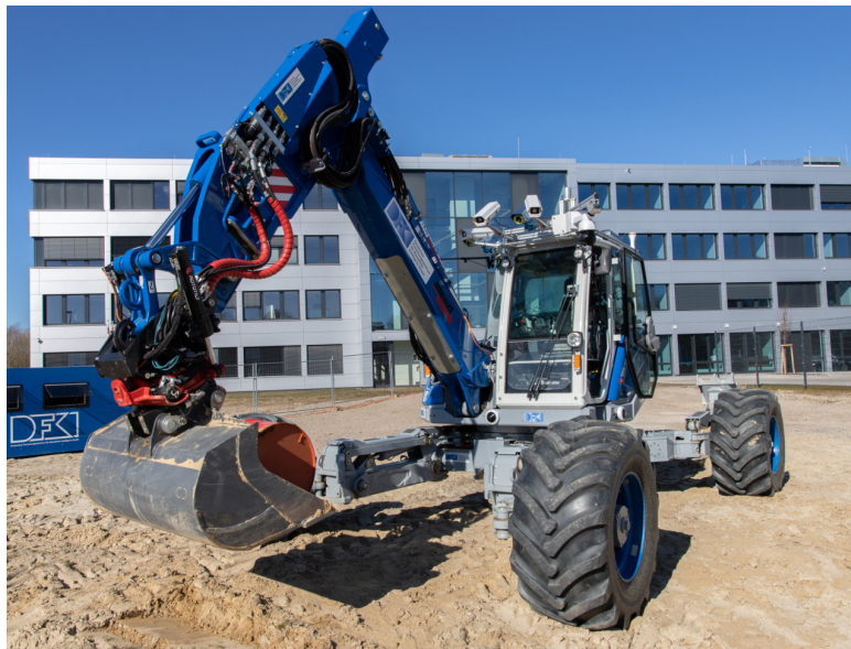
Figure 4.1: ARTER is a walking excavator robot being developed by DFKI.
