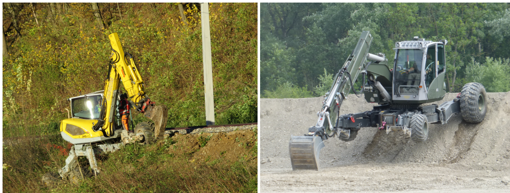
Figure 1.5: Walking excavator in extreme terrains where the wheeled-legged design is used to adapt to terrain (left 1 ) as well as using the manipulator on slopes (right 2 ).
