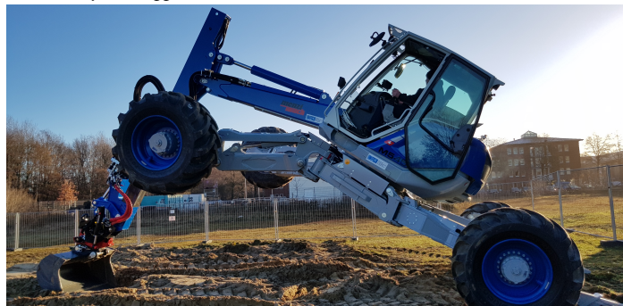
(c) ARTER ( Babu et al. 2024 ) is a walking excavator robot with adaptive legged wheels and a manipulator which can support locomotion.
