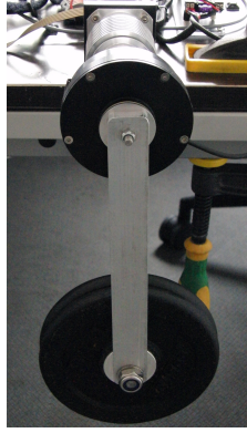
Figure 2.6: Calibration setup with the swinging mass for calibrating the model and estimating the hysteresis parameters.
