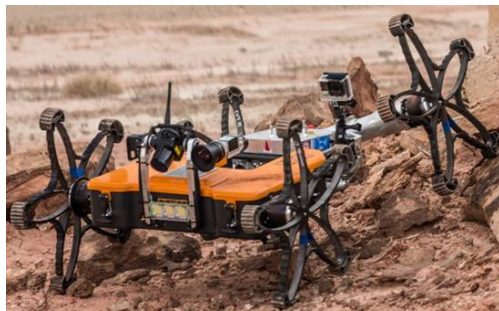
(a) The Coyote3 robot ( R. U. Sonsalla et al. 2015 ) is a passive hybrid robot with a hybrid legged wheel.
