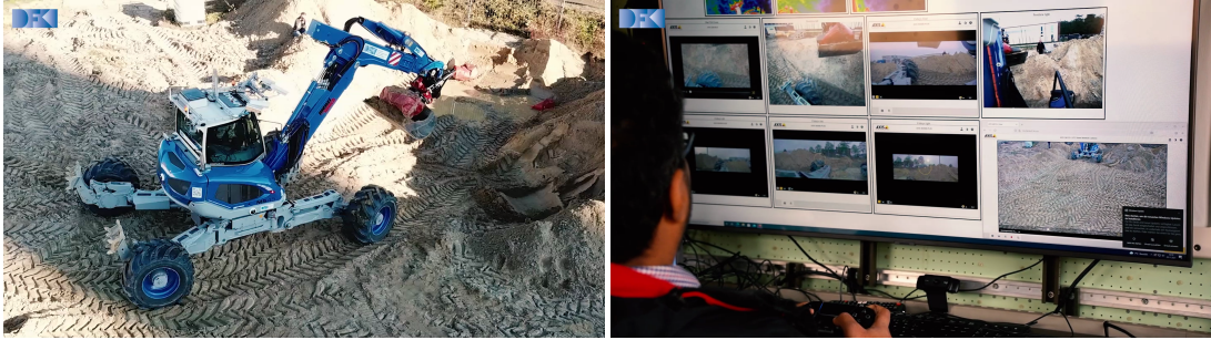
Figure 4.13: ARTER is used in this scenario to recover barrels from environments that are hazardous for humans. This is achieved using ARTER-MCS and remote-control, where the primary operator feedback is based on video streams.
