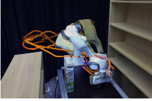
Fig. 10. Example of multimodal trajectories executed in the warehouse environment using MPD. Starting from the same joint configuration, the task is to reach an end-effector pose on the table while avoiding collisions with the environment. The orange lines depict the end-effector trajectories, and the overlaid images show the last frame on the trajectory. Our model generates multiple goal robot configurations for similar desired end-effector poses.
