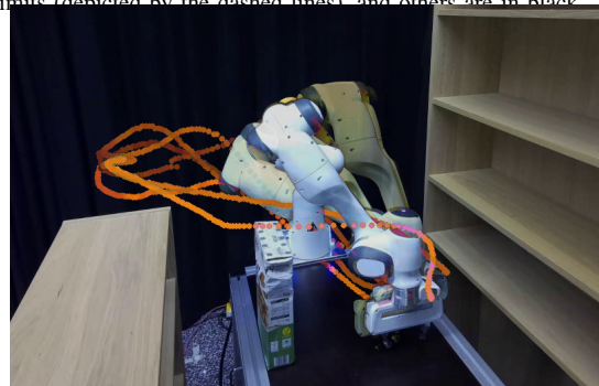
Fig. 10. Example of multimodal trajectories executed in the warehouse environment using MPD. Starting from the same joint configuration, the task is to reach an end-effector pose on the table while avoiding collisions with the environment. The orange lines depict the end-effector trajectories, and the overlaid images show the last frame on the trajectory. Our model generates multiple goal robot configurations for similar desired end-effector poses.
