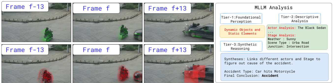
Figure 2: An example of the IMPACT framework processing a traffic incident. The pre-processing module uses the KFD algorithm to track keypoint trajectories (green lines) on the moving sedan and motorbike. As the vehicles converge, their intersecting vicinity circles (vc-circles, shown in red circles) and the resulting highlighted impact area (red box) trigger the detection of a critical event. The flagged \mathcal{F}_{seq} is then passed to the MLLM for hierarchical reasoning. The MLLMs output on the right-hand side is a structured analysis comprising Tier-1 (Perception), Tier-2 (Description), and Tier-3 (Causal Reasoning), providing a comprehensive understanding of the accident.
