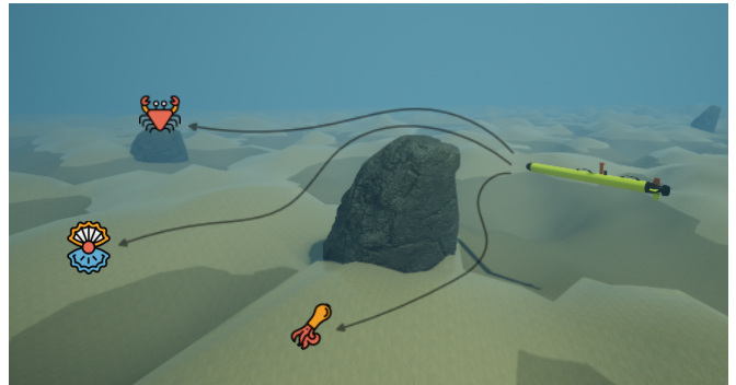
Fig. 1: The navigation task is simulated in HoloOcean. For the specified species in each task, the AUV should navigate to find the crab, the shell or the octopus.
