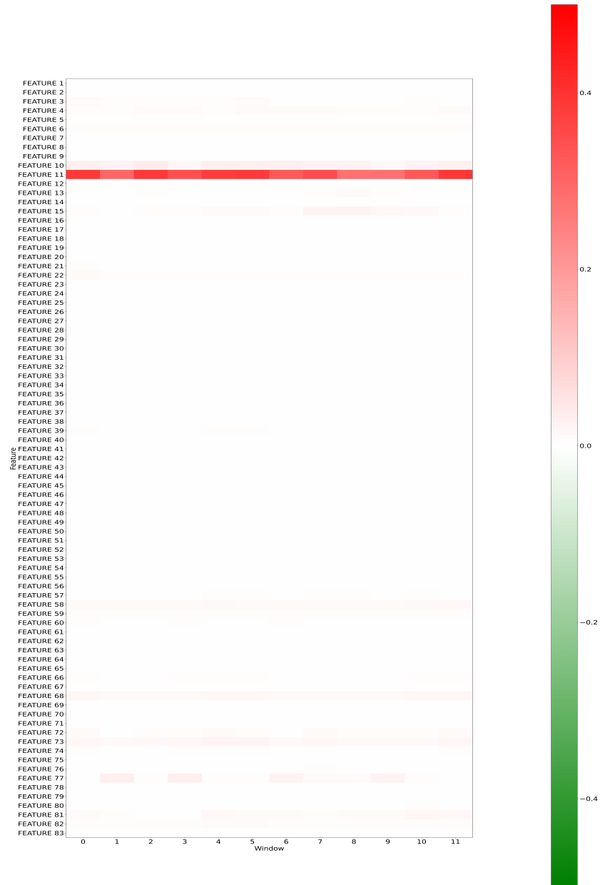
Fig. 9: Signal dropout anomaly on Feature 11. Feature 11 is affected by a synthetic signal dropout anomaly, where the signal abruptly drops to zero over the affected interval, and the attribution pattern correctly highlights the anomalous feature.
