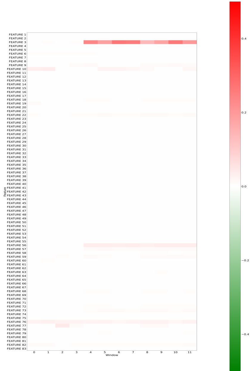
Fig. 8: Saturation anomaly on Feature 3. Feature 3 exhibits a synthetic saturation anomaly, in which the signal is clipped at a limit, and the anomaly is correctly identified.
