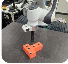
(c) Push-T real-world setup, with a FR3 arm, custom end-effector, and Mocap markers.
