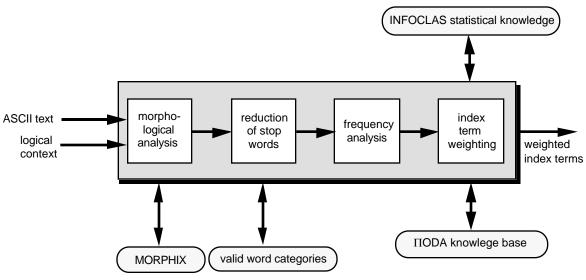
Figure 6: Components of indexing module.
