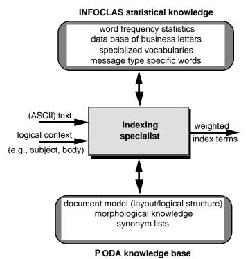
Figure 5: External interface of indexing module.
