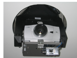
Figure 1: Steerable projector and camera unit ( Fluid Beam )
