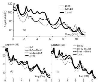
*Figure 2:* (a) Linear prediction (LP) spectra of the mid-frame of /aI-aI/ diphone in soft, modal, and loud databases, (b) LP spectra of the mid-frame in soft, modal, soft-to-modal, and modal-to-soft databases, (c) LP spectra of the mid-frame in modal, loud, modal-to-loud, and loud-to-modal databases.
