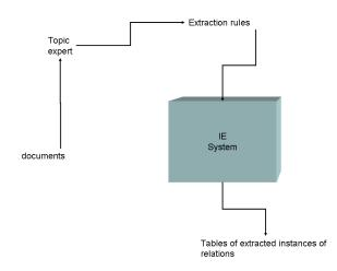
Figure 1: A hand-coded rule–based IE–system (schematically): A topic expert implements manually task–specific extraction rules on the basis of her manual analysis of a representative corpus.
