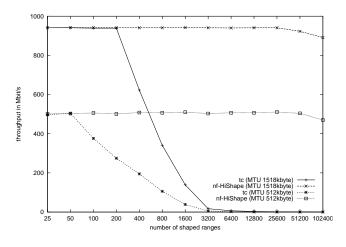
Figure 1: *nf-HiShape* is able to handle more traffic than *tc* on large sets of shaping rules
