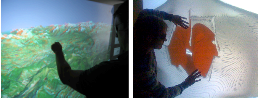
Figure 5: Two examples of applications interfaced by the iMUTS interaction paradigms. (Left) a user interacts in a landscape-planning scenario on an FTIR multi-touch wall with an anaglyph-based stereoscopic projection. (Right) a user performs volume deformation in a medical scenario using a large FTIR-based passive back projection iMUTS.
