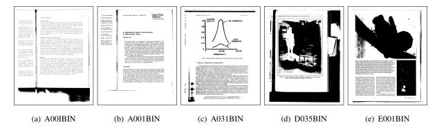
Fig. 1. Sample images from the University of Washington Database 3 (UW3). The samples illustrate the variability and unpredictability of marginal noise in UW3. Across the entire database, noise outside the page margins of the scanned page consists of connected components at many different sizes and shapes, including actual text, and ranges from nearly absent to dominating the image. On other pages, illustrations outside the text area may resemble marginal noise and black borders.
