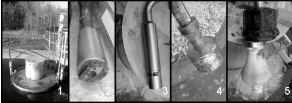
Figure 2 1 = floating decant device with mountings for 2, 3, 4 and 5; 2 = TSS probe; 3 = NO 3 -N probe; 4 = SL probe; 5 = SV probe (all devices from HACH LANGE GmbH)
