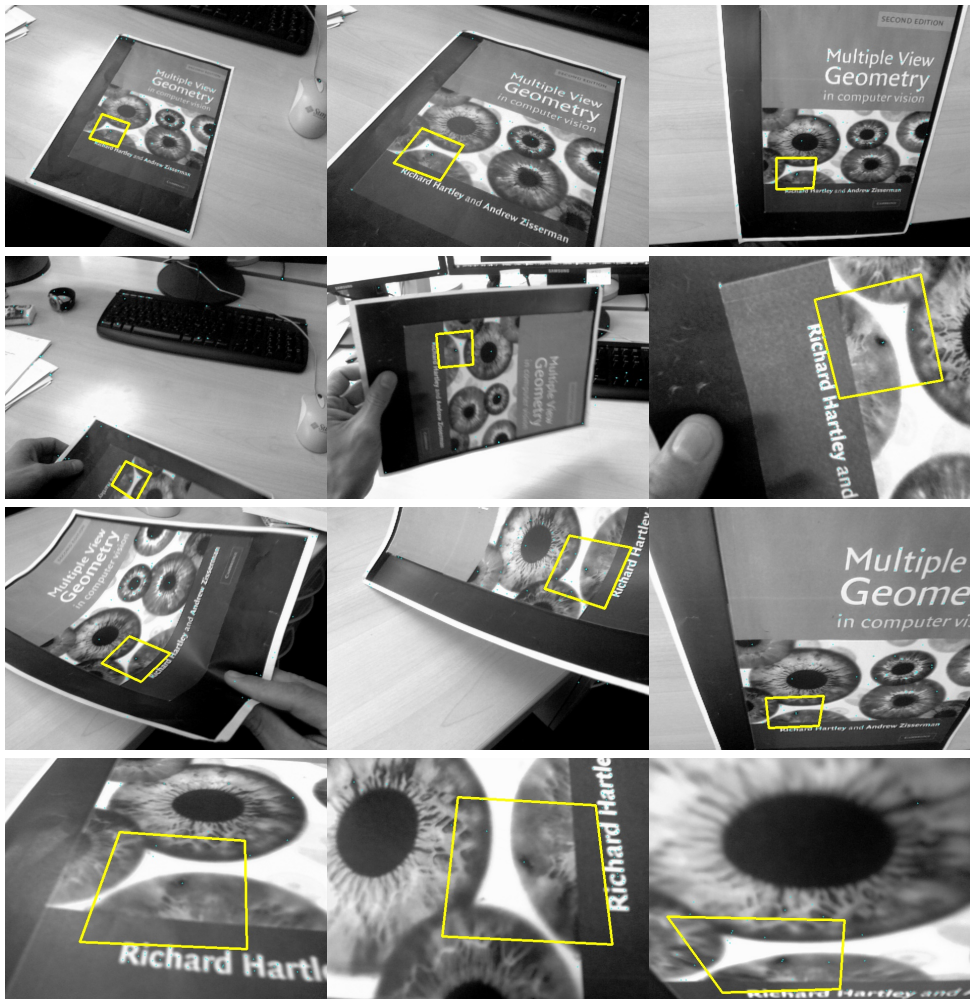
Figure 6: Estimation of the local patch transformation. Our system detects the learnt point and estimates its pose in real time, even in presence of large scale variations. A full video is available on the authors' website at http://av.dfki.de/~pagani .
