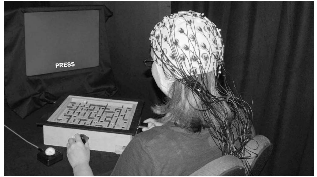
Fig. 1. Experimental setup: Subject is playing BRIO ® and is reacting towards rare target stimuli (alerts) by pressing a buzzer.
