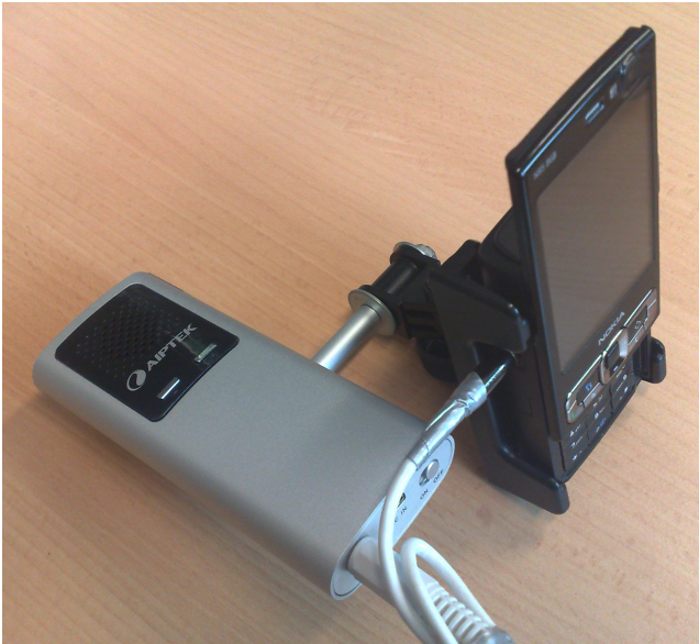
Figure 3: The Prototype used for ShelfTorchlight : Nokia N95 8gb and an Aiptek T30
