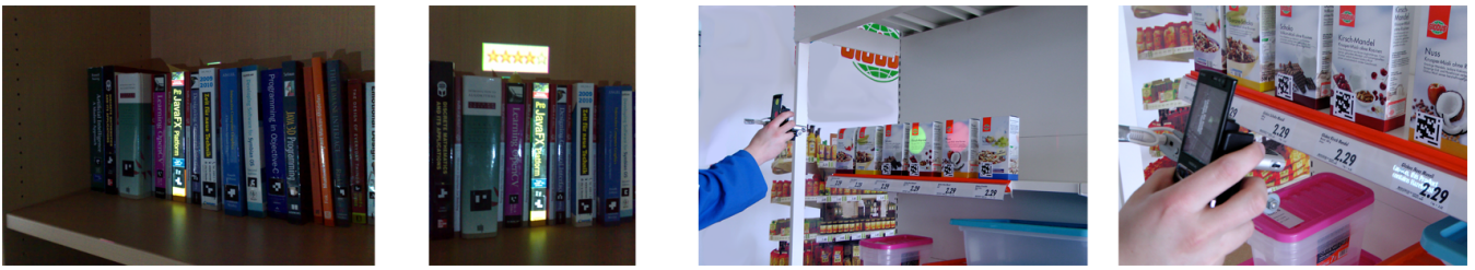
Figure 2: Interaction techniques of ShelfTorchlight application: (Library Scenario) The book a user is searching for gets highlighted (left) or the rating of the book gets projected beside the book (middle-left). (Retail Scenario) Onto the facing of the product the user gets a projection on how suited a product is taking his personal profile into account (middle-right) and the semantic zoom reveals the reason for the classification (right).
