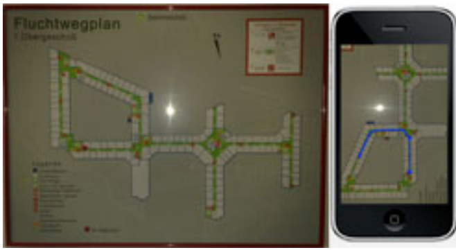
Figure 1: Left: An example of an indoor "You-Are-Here"-map (This photo was taken at the -removed for blind review-). Right: Position visualization on an iPhone on the basis of the You-Are-Here-map using our compass dead reckoning approach.
