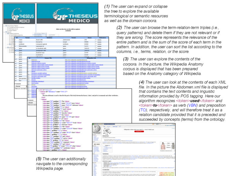
Figure 6: (1) First view that the clinician sees from the browser. The tree on the left reveals the contents available for browsing. (2) Second view of the browser that displays the query patterns as a sortable list. (3) Anatomy corpus files with links to original Wikipedia files. (4) Wikipedia Abdomen.xml with POS tagging. (5) Corresponding page in Wikipedia.
