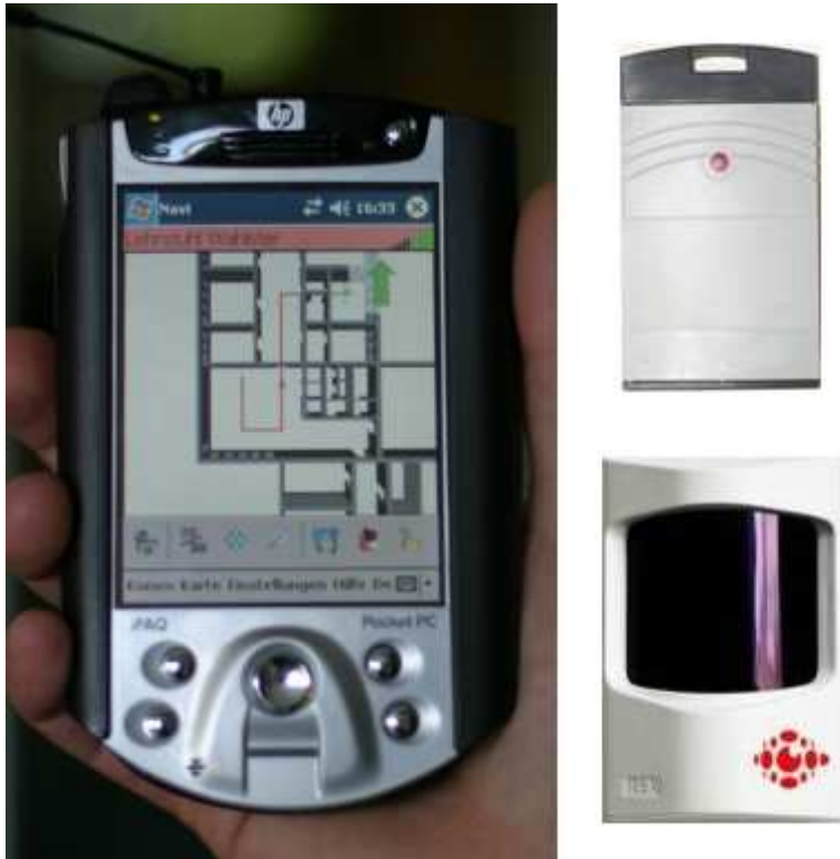
Fig. 2. iPAQ with attached RFID sensor and built-in infrared sensor (left). Active RFID tag and infrared beacon (right).
