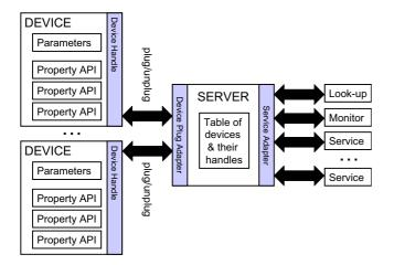
Figure 2: Architecture of the plugboard
