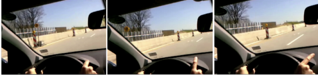
Figure 1: A sequence of images taken from a video showing a person executing a clockwise circular gesture while driving. The video was taken without a functional gesture recognition system in a standard car in order to illustrate the intended functionality.
