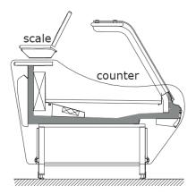
**Figure 3**: The figure shows the illustrated application setup with the counter, the scale with display for employee and customer and the Kinect mounted above the counter.
