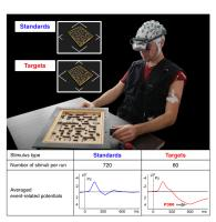
**BRIO Oddball paradigm:** Experimental setup to evaluate methods for single-trial P300 detection
