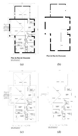
Figure 2: Original floor plan (a), the detected thick walls (b), the intermediate image after wall segmentation (c), and the image after thin line removal (d).
