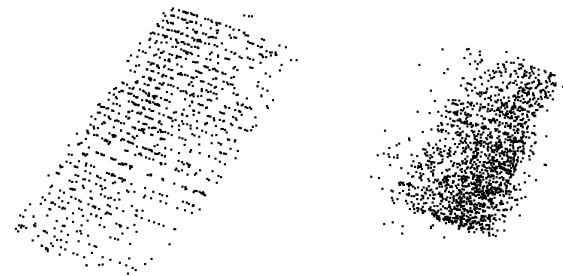
Figure 4. 3D reconstruction of book page with RANSAC. Left side shows the proposed method. Right side shows default matching.
